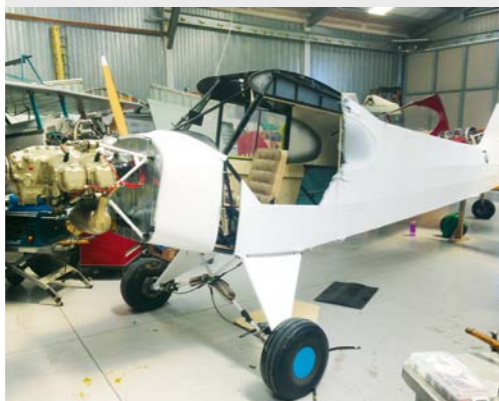
90hp Cub Bkx during rebuild / rebag.
