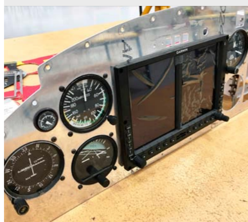
Garmin G500 installation
